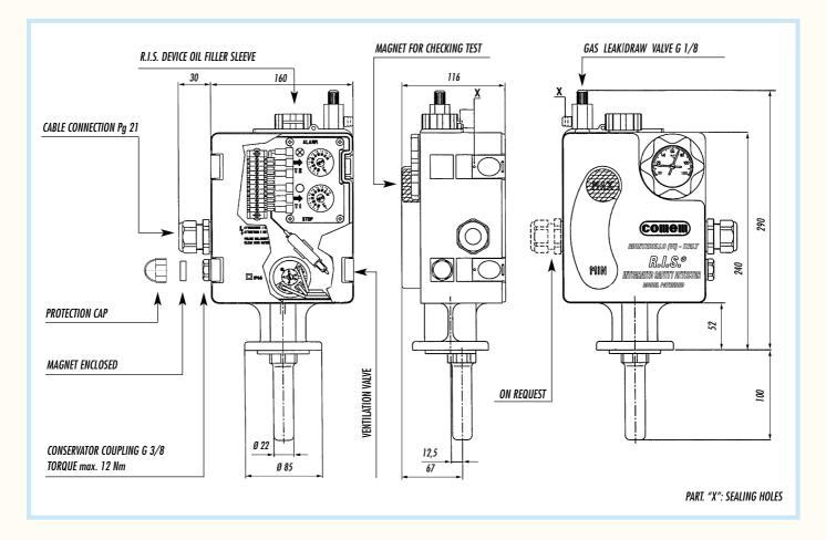
It is composed of a robust plastic body, watertight and resistant to extreme climates, that houses a series of instruments and keeps under constant control the following operating conditions of the transformer:
